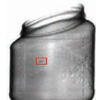
Detect defect side wall inclusions in glass containers
